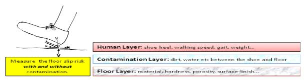
SlipAlert helps you measure the slip risk of the floor with/without contamination. You can manage factors in each layer to ensure the floor is suitable for its use... i.e. in a kitchen staff can wear safety shoes, on a hospital ward the floor can be kept clean/dry. For a hospital corridor it is important to understand the level of risk when the floor is in use and before/after cleaning.
